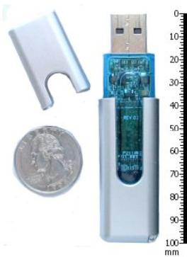
Another popular option is the USB “flash drive,” which can store up to 2 GB of data (There are one billion bytes in a gigabyte [GB] and one million bytes in a megabyte [MB].) It is a very small removable storage device that plugs into any computer with a USB outlet and functions like a computer drive. Files can easily be saved to and removed from the drive by dragging and dropping.
